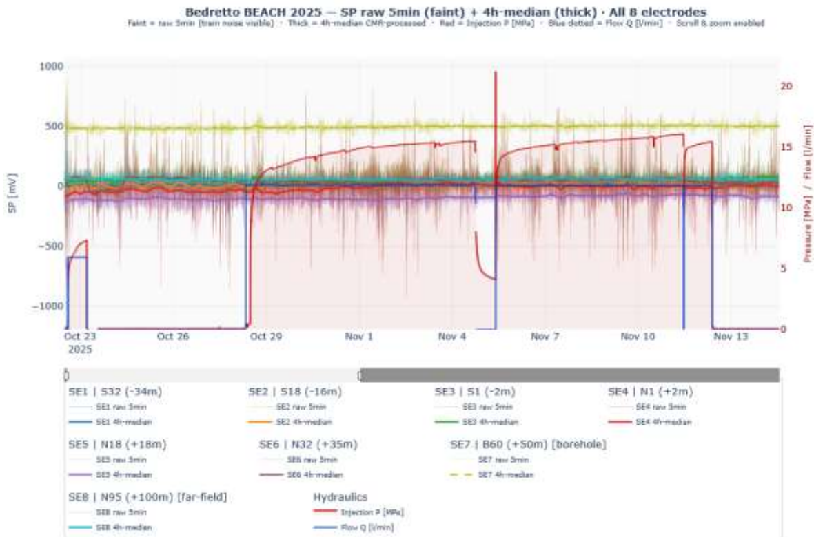
Figure 1-2: Overview of the BEACH self-potential dataset showing raw SP signals (5 min median, faint lines) and 4 h median SP signals (thick lines) for all eight electrodes. Injection pressure (red) and flow rate (blue) are shown on the secondary axis.
