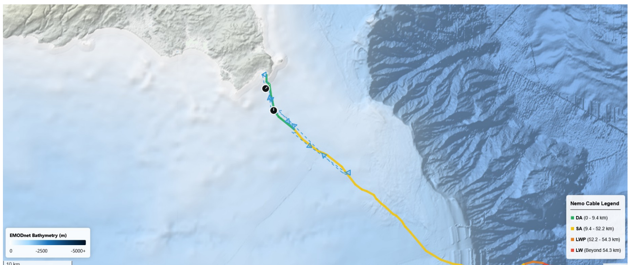
Figure 2: Bathymetric map of the INFN-LNS installation site indicating the location of the submarine cable, the trajectory of the vessel and the location of the hydrophone deployments.
