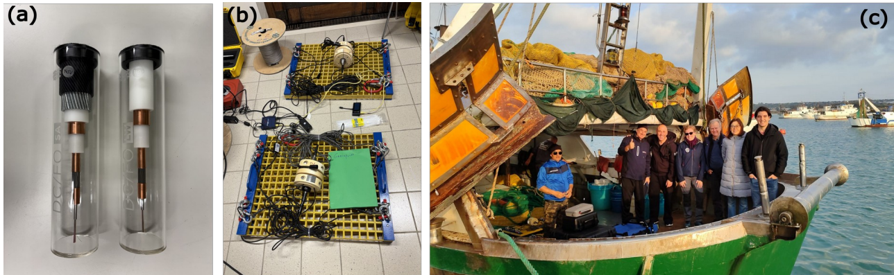
Figure 1: (a) Double-armoured and single-armoured structure of the submarine fiber-optic cable, (b) deployment structure for the piezoelectric hydrophones, and (c) FREDAS team onboard a commercial vessel at the port of Portopalo di Capo Passero, Italy.
