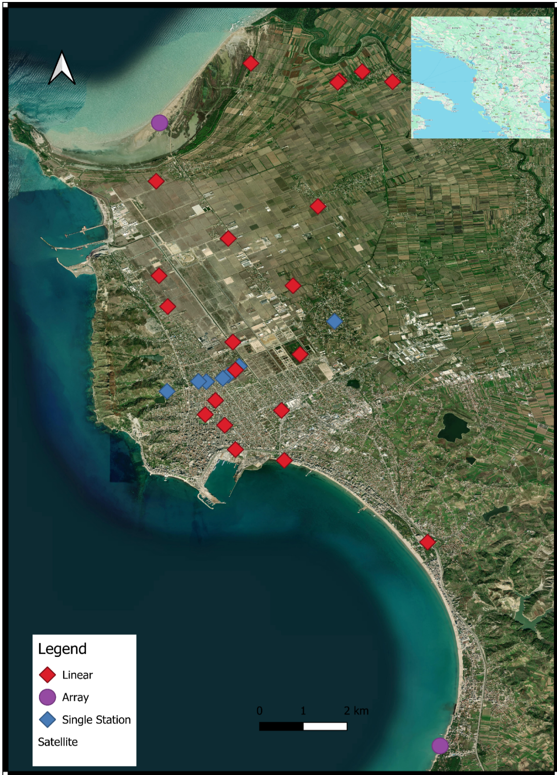
Figure 1. Distribution of measurement sites in the Durrës basin, including liquefaction-observed sectors, critical infrastructure sites and representative basin transects.
