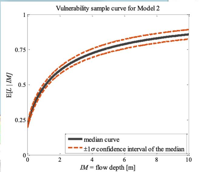
Vulnerability curve based on data for the Chilean Tsunami 2010.
