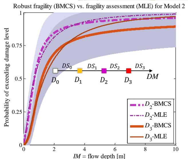
Fragility curves for non-engineered light timber damaged due to 2018 Sulawesi-Palu tsunami
