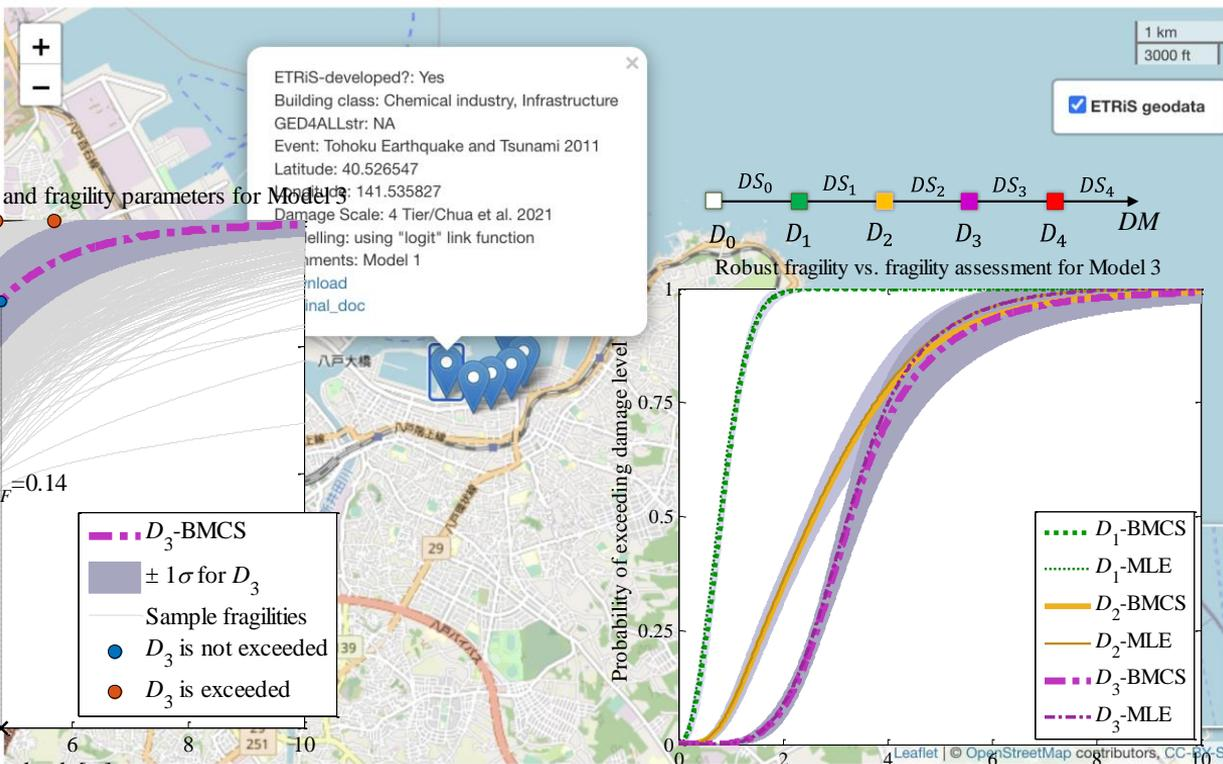
Fragility curves for Chemical Industry Infrastructure Damaged due to 2011 Great East Japan earthquake and tsunami
